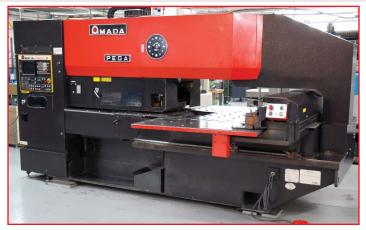
**AMADA** 22 Ton Turret Punch, Model PEGA 244, Fanuc 6 M Control, Travel: X & Y-40", Table Speed: X & Y-2000 IPM, 40" x 40" Table Size, 49" Throat, 30 RPM Turret Speed, 24 Station Turret, 350 T/Min Stroke Per Minute, .236" Max Sheet Thickness, 3.5" Max Hole Diameter, 40" x 40" Sheet Size, 40"x80" With Repositioning, s/n P2440358
