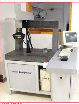
LASER DESIGN LASER CMM. MODEL SURVEYOR 1200
