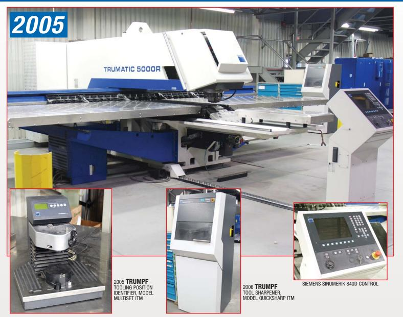
2005 **TRUMPF** 24 Ton Turret Punch, Model Trumatic 5000R-1600, Travel: X-118.11" & Y-64.96", Working range: X- Minus 1.96" To Plus 120.86" & Y-Minus .275" To Plus 65.35", Maximum Axis Speed: X-328'/Min , Y-196'/Min & C-330 Revolutions/Min, .314 Max Sheet Thickness, 3" Max Tool Diameter, 21 ATC, Siemens Sinumerik 840D Control, Only Approx. 5,000 Hours, Light Curtains, 460V, s/n T-9749 - A0060A0458, Plus Assorted Trumpf Tooling
