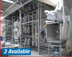
TWO STAGE RAINFALL TYPE INVESTMENT COATING CHAMBERS, PLUS DUAL ELEVATOR DRYING SYSTEM
