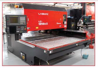
1995 **AMADA** Laser, Model LC-1212 $\alpha$ II, Fanuc Oscillator Laser, Model C1500B, 1,500 Watts Max Laser Output, 50"Axis Travel, 65'/Min Cutting Speed, Rapid Axis Speed: X & Y-262'/Min & Z-196'/Min, 50" x 100" Max Sheet Size, .354" Max Sheet Thickness, 462 LBS Max Work Piece Weight, Fanuc Series 16-L Control, s/n 11212251
