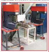
PEMSERTER 6 TON RIVETING MACHINE, MODEL 4
